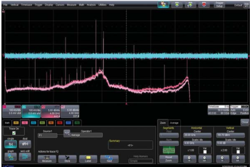
Figure 5: Noise density of a frequency interleaved oscilloscope (notice the noise spike around 15 GHz and 30 GHz)
